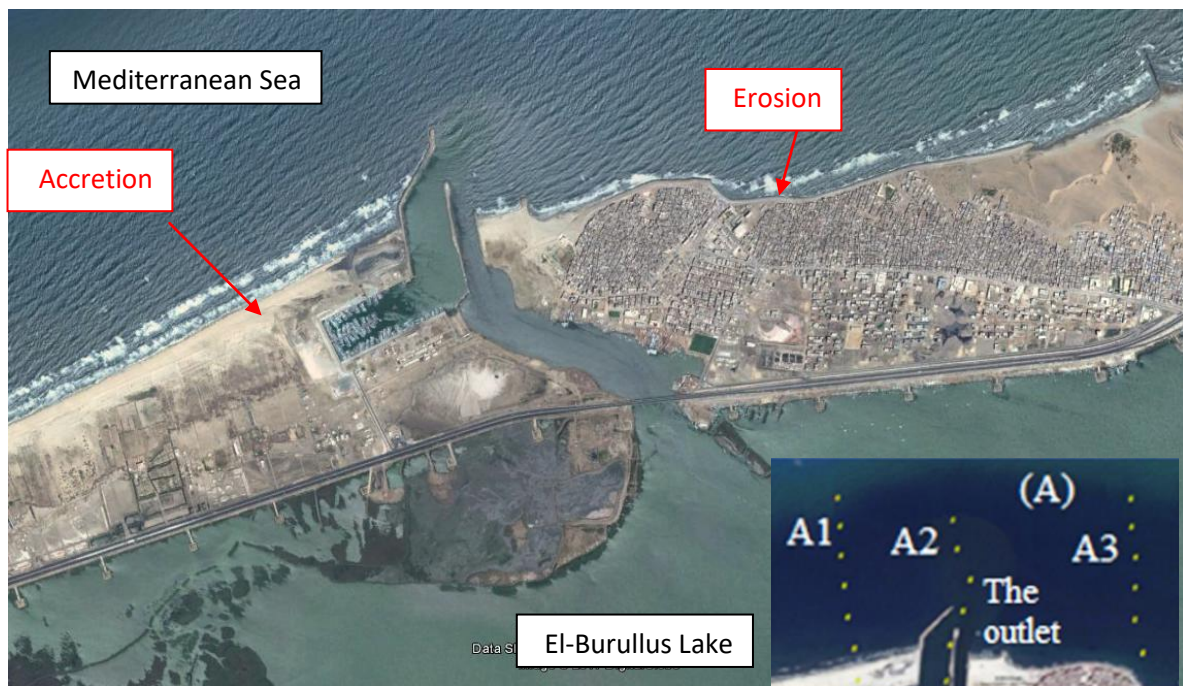
Figure 5. El-Burullus Lake outlet with erosion and accretion
