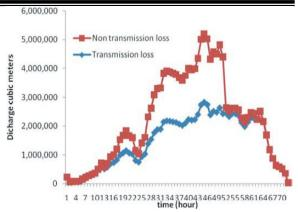
**Fig.7:** The simulated runoff hydrograph for Wadi Al Rimah using the entire flow contributing areas (i.e. time zones) and the distributed rainfall of Fig. 5 A. (Note :the impact of transmission loss on the hydrograph peaks and attenuations).
