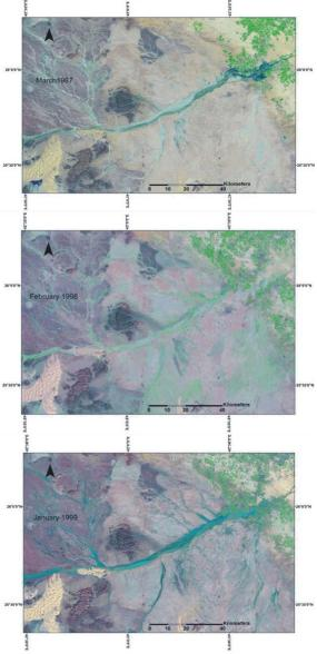
**Fig. 3:** Distribution and extent of active channels and flash floods based on the Landsat images, March 1987 (top), February 1998 (middle) and January 1999 (bottom)
