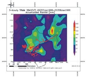
**Fig. 5 A:** TRMM estimated total rainfall(mm) and distribution over Wadi Al Rimah catchment on the V<sup>th</sup> of January 1999. Note: the correspondence between the rainfall pattern and the resulting active channels (red lines), which are digitized from the Landsat image acquired shortly after this rainfall event (Fig. 3)
