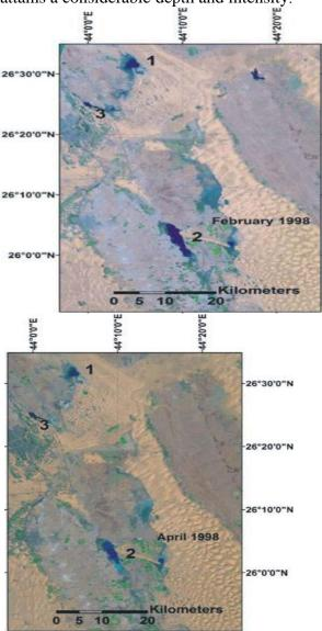
Fig. 6: The resultant water ponds of the flash flood of January 1998 (Note: the changes of surface extent between February and April 1998. The stored water volumes in ponds 1, 2 and 3 were computed using these delineated surface areas and the dry-bottom topography derived from the SRTM)
